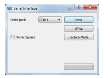
The serial interface icon brings up a dialog that allows the configuration to be downloaded/uploaded from the radio. If the radio rejects any of the parameters that are written, the "Complete" message will be replaced with a warning.
