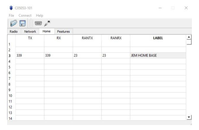
• **Home Channels** – This table is used to configure the AAR channel numbers along with the RAN codes that are assigned to each home number (1 – 500).
