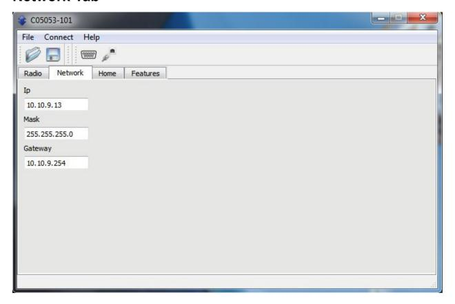
• **Network parameters** – These set the IP address of the radio. If these are changed, the radio must be restarted before it will use the new values.
