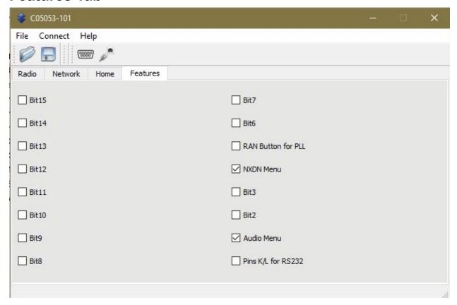
Users can limit functionality of the JEM Radio II when installed in a locomotive by deselecting an option on the **Features** tab.
