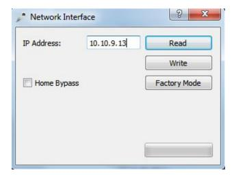
The network interface icon brings up a dialog that allows the configuration to be downloaded/uploaded from the radio if it's on a network. It functions identically to the serial interface dialog.
