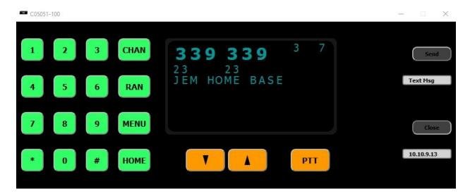
The normal display will show the 6-digit AAR channel number in enlarged print. The home channel number and channel label (if there is one) along with the volume. The home channel label is displayed on the 4th line. This is also where digital messages are displayed as well as RAN code and HOME channel entry prompts.
