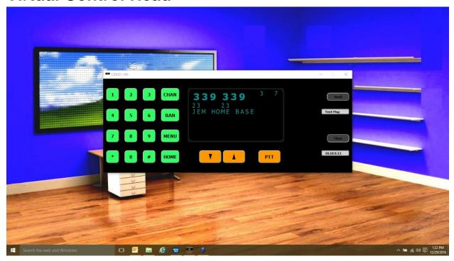
A command can be sent to the radio that will cause it to send all the data that gets sent to the display to also get sent out the PC port serial port or the Ethernet port. This makes it possible to write a software application that can display the data as well as send button press commands to the radio essentially making it a software equivalent of the control head.
