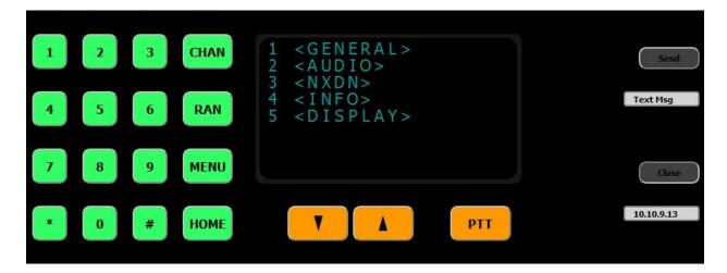
The MENU key will bring up a list of options that can be selected with the number keys. Once the option is selected, the value can be incremented or decremented by using the volume control button. When menus are displayed, pressing the menu key again will exit the current menu section. Pressing the CHAN, HOME, or PTT button will also exit menu mode. See (Appendix E) for the menu hierarchy.
