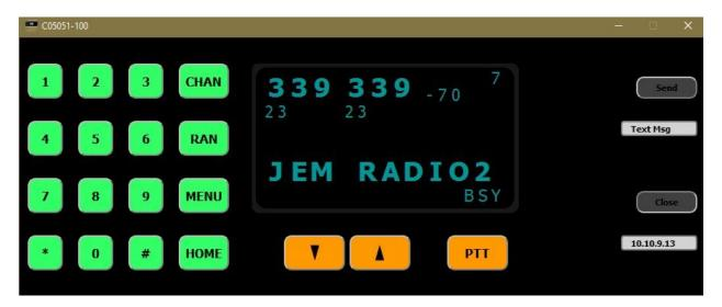
When a reception is received from another radio, the RSSI value will be shown near the top-right corner, just below the volume setting. The abbreviation "BSY" will be displayed in the lower right corner.
